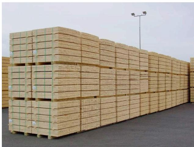
**Figure 3** Well built stacks of banded sawn timber packs
