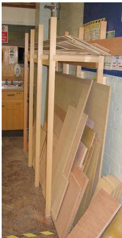
Figure 5 Small racking system
